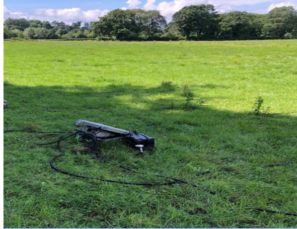
MT recorder and sensors/wires
